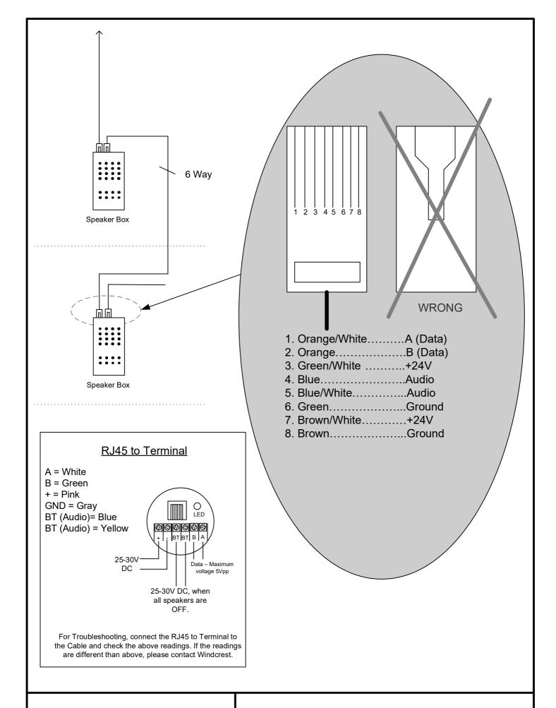
RJ45 Plug & RJ45 Plug to Terminal
