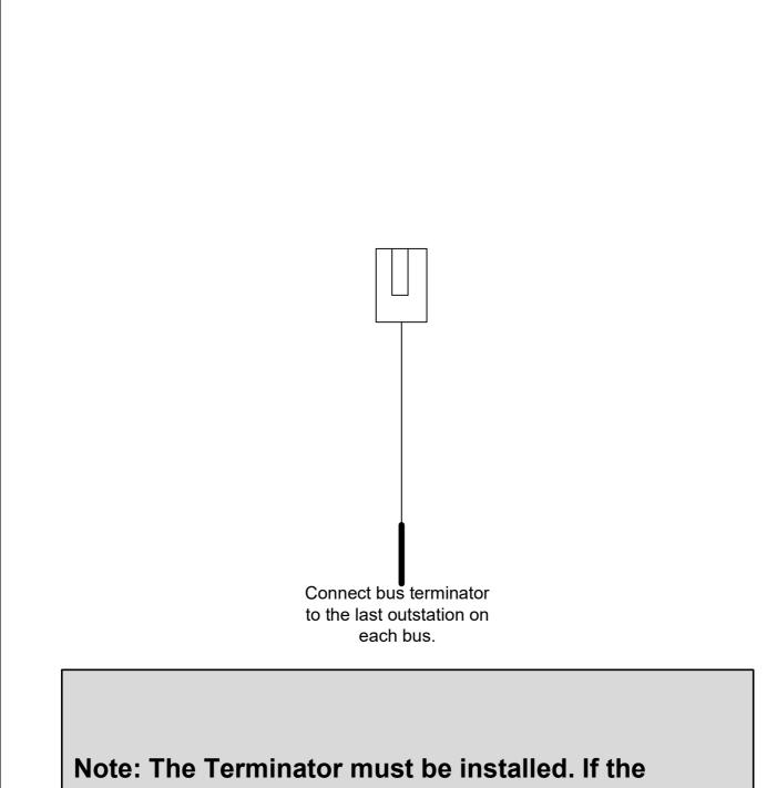
Note: The Terminator must be installed. If the terminator is not installed it will result in un-reliable operation of the system due to data corruption.
