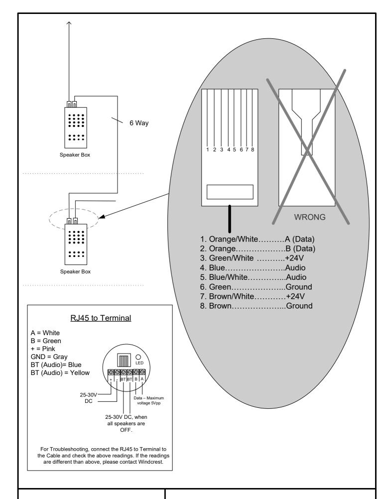
RJ45 Plug & RJ45 Plug to Terminal
