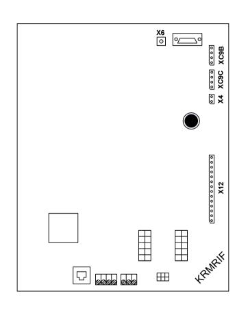
KONE KRM Existing Factory Arrangement in the Top of Car Connection Box (Kone Dg No.812301E24)
